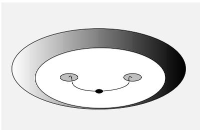
The thermocouple is well protected while the TC head is in the instrument. Cleaning procedures detailed in this manual should not harm the thermocouple, but it can be deformed or broken if contacted by any object while it is out of the instrument.
