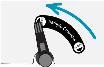
1 Verify that the sample chamber lever is in the open position.
