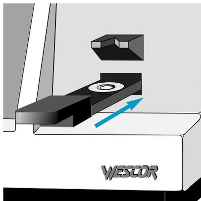
**7** Gently push the sample slide into the instrument until it stops. (Never close the chamber unless the sample holder is in this position.)
