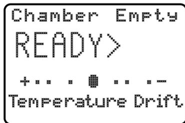
While the instrument compensates for small changes that occur over time, moving the instrument to a different area or exposing it to too much air circulation will shift the osmometer's reading and calibration points. The Temperature Drift scale allows you to determine when internal temperature has stabilized.
