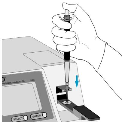
**4** With the pipettor tip resting in the notch of the pipettor guide, position the tip about 5 millimeters above the center of the sample disc.
