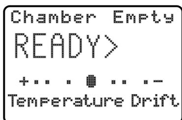
When the instrument is not in use, leave the cleaned sample holder empty and locked in the measurement position. If the chamber is left open for longer than 2 minutes, a warning chime sounds.
