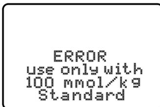
If you run the Clean Test and the display shows "ERROR Use only with 100 mmol/kg standard," this may indicate that you incorrectly used a 290 mmol/kg or 1000 mmol/kg standard for the test. Run the Clean Test again using the 100 mmol/kg standard.
